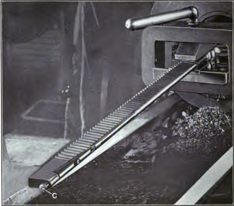
FIG. 144.—Showing the wedge adjustment.
